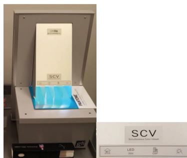
Figure 2: GTI Simultaneous Color Viewer (left). Icon labels for SCV light sources (right).
