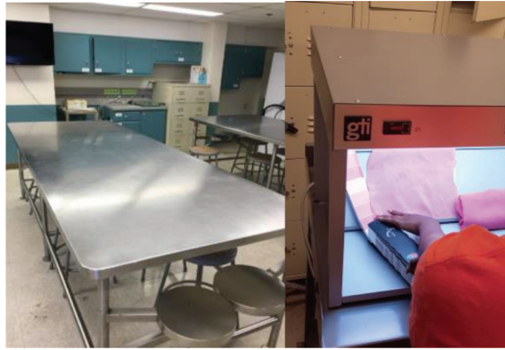
Figure 11: Lighting conditions in study of sample color matching – ambient classroom lighting (left) and Color Matching Booth (right)
