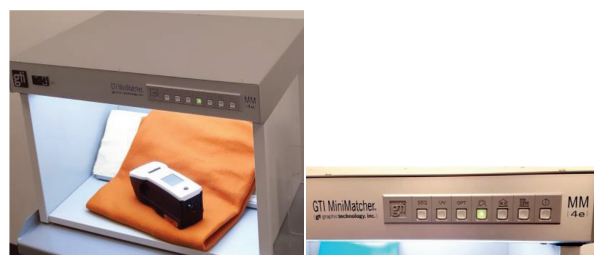
Figure 4: GTI MiniMatcher MM-4e Color matching Booth (left). Light source switches with icon labels (right).
