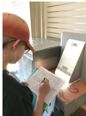
Figure 10: Simultaneous Color Viewer used in studies on effect of lighting on sample color.
