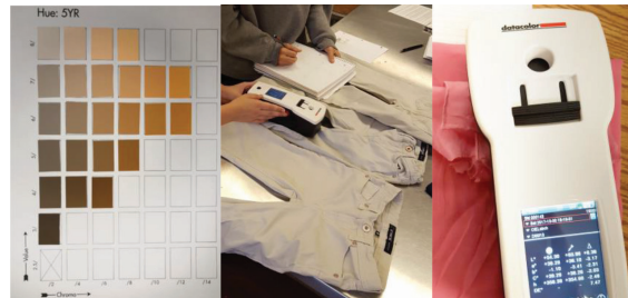
Figure 7: Color measurement exercises completed using the handheld spectrophotometer: 1). Measuring adjacent colors on a Munsell hue chart (left). 2). Measuring color differences of ready-to-wear products (middle). 3). Measuring color differences of fabrics with same fiber content but different fabric tie dyed in the same dye bath (right).
