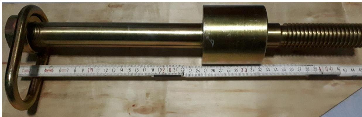
Fig. 1 Tree house attachment Bolt (TAB)
