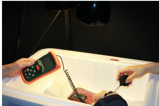
Figure 7. Researchers utilizing a light meter and a temperature probe to check settings on the raw ground beef package.
