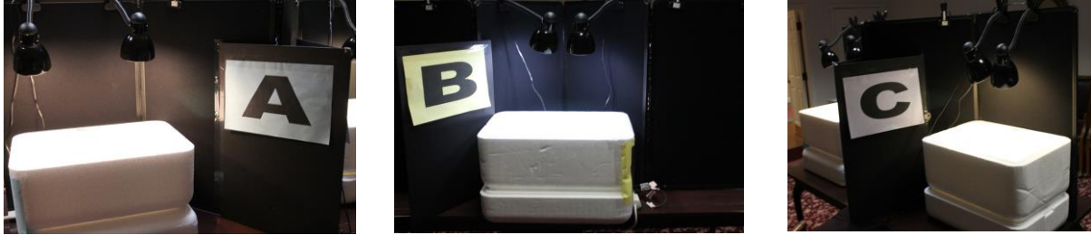
Figure 6. Three lighting treatments (LED - warm, LED - cool and compact fluorescent,) illuminating raw ground beef packages in styrofoam ice chests
