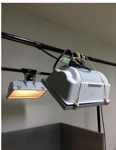
Figure 1. 1500 watt quartz halogen and visual acuity test scoop fixtures
