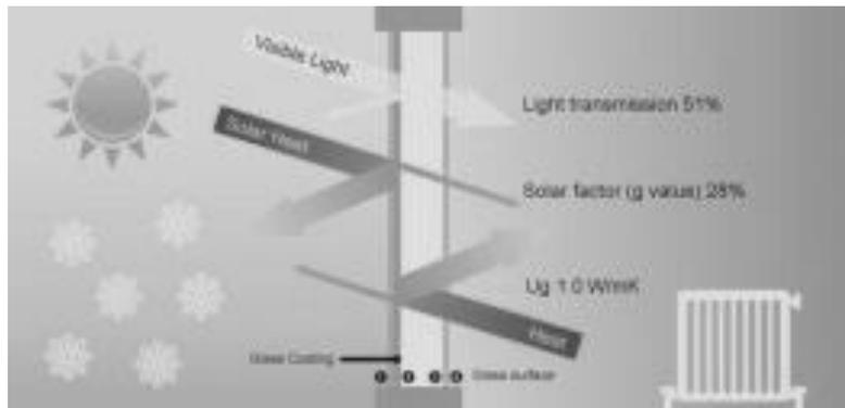
Figure 9: Sun Guard Super Neutral SN 51/28 Tech Specification provided by Guardin
