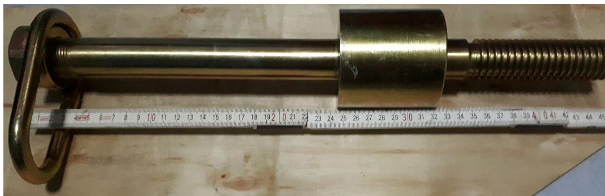
Fig. 1 Tree house attachment Bolt (TAB)
