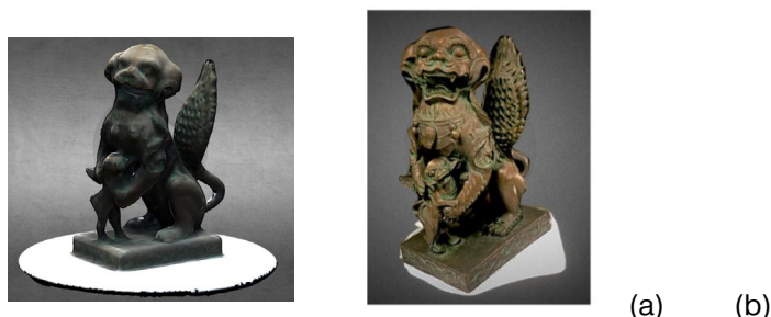
Figure 14. (a) Foo Lion, Hand-held scanner (b) Foo Lion, ReCap Autodesk Photogrammetry Scan
