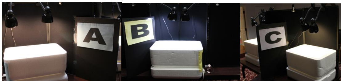
Figure 6. Three lighting treatments (LED - warm, LED - cool and compact fluorescent,) illuminating raw ground beef packages in styrofoam ice chests
