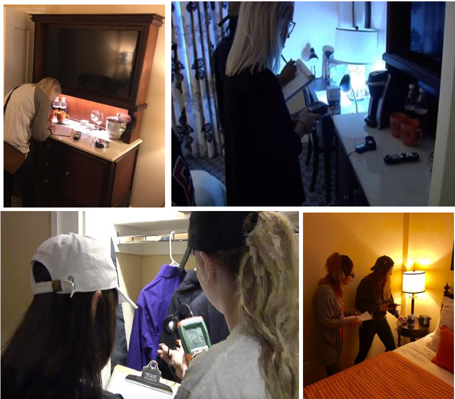
Figure 5. Student measurements of hotel room lighting parameters and documenting proposed changes in sketches for design variants
