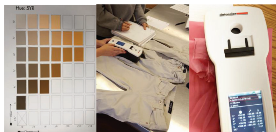
Figure 7: Color measurement exercises completed using the handheld spectrophotometer: 1). Measuring adjacent colors on a Munsell hue chart (left). 2). Measuring color differences of ready-to-wear products (middle). 3). Measuring color differences of fabrics with same fiber content but different fabric type dyed in the same dye bath (right).
